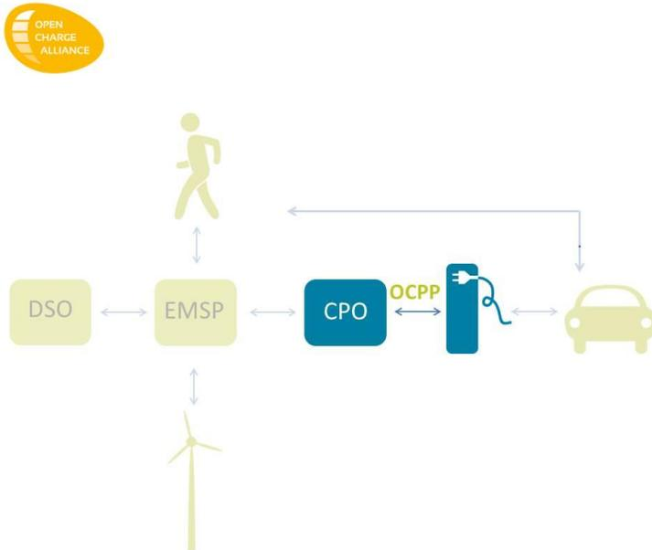
Figure 1: Architecture and Generic Implementation of Open Charge Point Protocol
