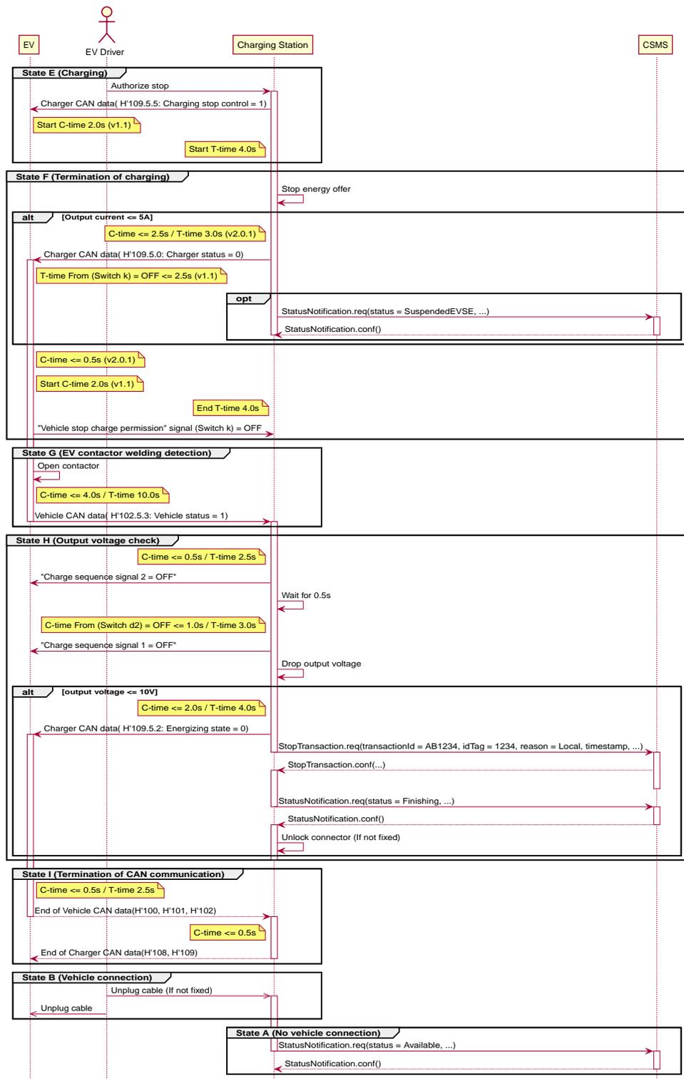
Figure 8. Sequence diagram: Stop by Charging Station
