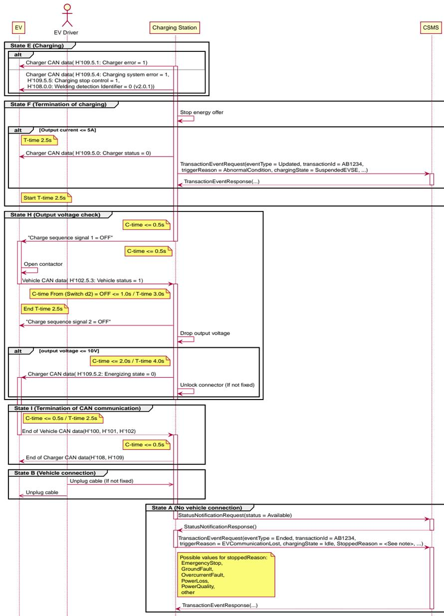
Figure 3. Sequence diagram: Stop by Charging Station (abnormal)
